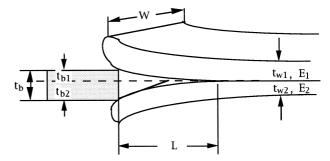
Fig. 2. Schematic of crack-opening method to determine bonding or surface energy.
