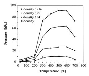
Fig. 9. Pressure increase in cavities after hydrophilic bonding and annealing at specified temperatures for 70 h [31].
