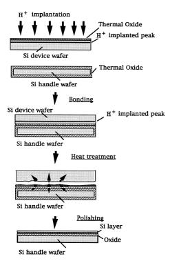
Fig. 10. Schematic of hydrogen-implantation induced layer splitting ('smart-cut') [17,39].
