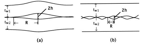
Fig. 5. Schematic of surface waviness.
