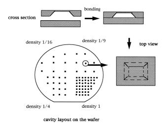
Fig. 8. Cavities used for measuring pressure increase due to interface reactions. (a) Schematic of test structure cavity. (b) Cavity layout on the wafer [31].
