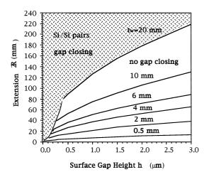
Fig. 6. Calculation under which conditions gap closure does or does not occur for different assumed wafer thicknesses from 0.5–20 mm and  $\gamma = 100 \text{ mJ}/\text{m}^2$  [17].
